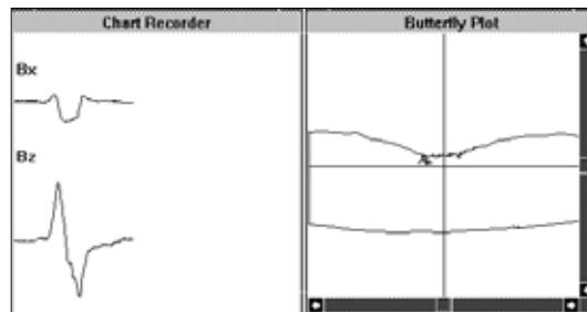
Figure 2. Example of chart recorder and butterfly plots from a defect
