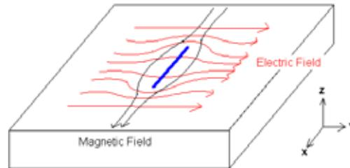
Figure 1. Definition of field directions and co-ordinate system used in ACFM
